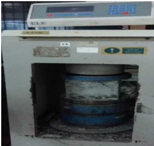
Fig. 2.9. Compressive Strength Test
