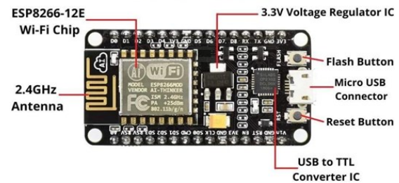
Figure 5: NodeMCU Parts
