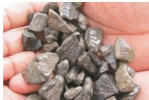
Recycled aggregate obtained after processing.
