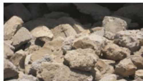
Demolition waste before processing
