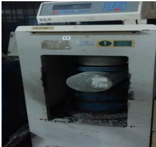
Fig. 2.10. Split tensile strength Test
