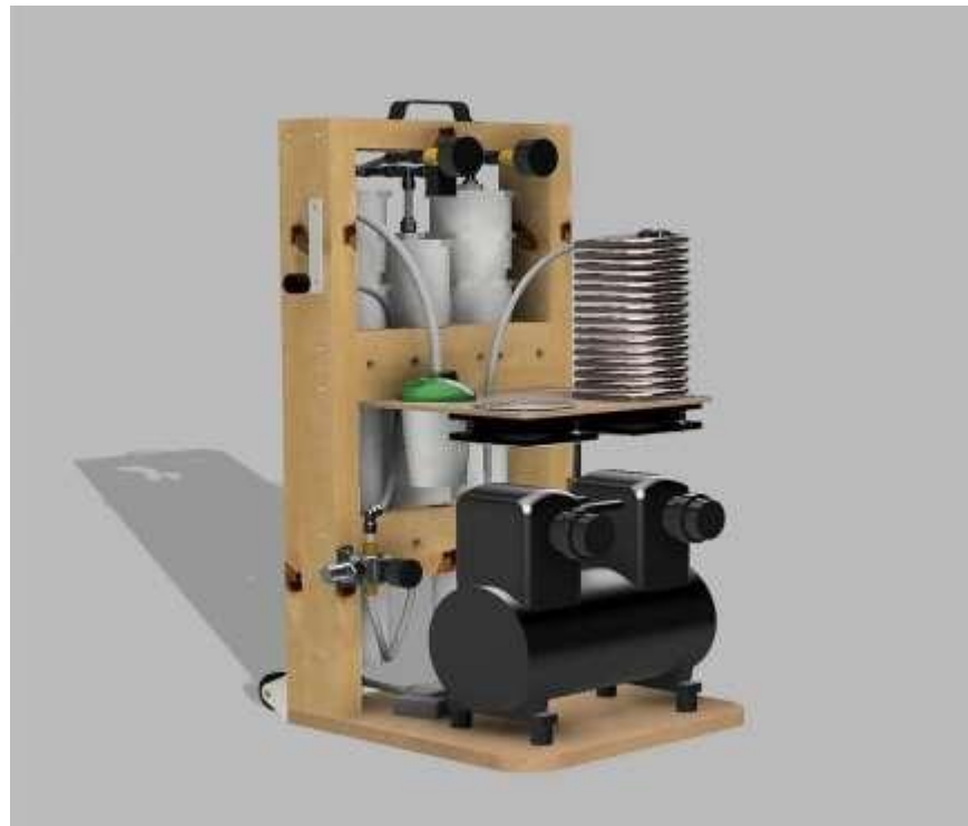
Fig 4.2.2 Isometric view of oxygen concentrated assembly
