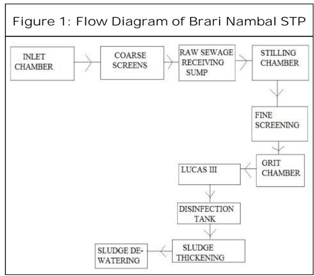
**Biological Treatment:** The main pollutants in the sewage are represented in the form of biochemical oxygen demand and chemical oxygen demand, ammoniacal nitrogen, nitrate nitrogen and phosphorus present also represent as polluting substances. The bacterial ability to utilize the harmful products and turn them into carbon dioxide and water molecules is utilized to treat the raw sewage.
