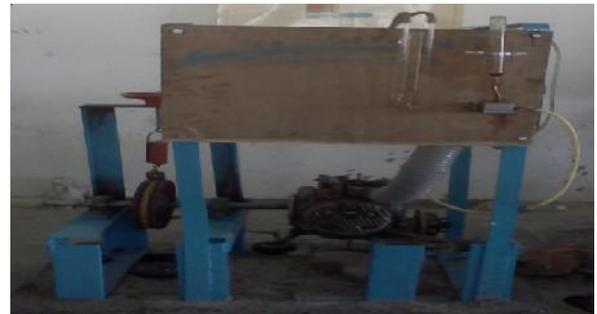
1 lists some of the important specification of the engine under test. The schematic layout of the experimental set up is shown in Figure 1. Fuel consumption was measured by using a calibrated burette and a stopwatch with an accuracy of 0.2 sec.
