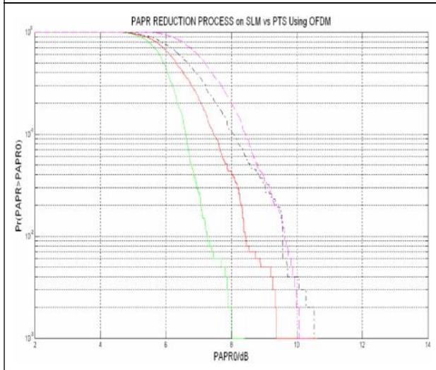
Figure 5: PAPR Reduction Using 64 Subcarriers in MIMO OFDM Systems
