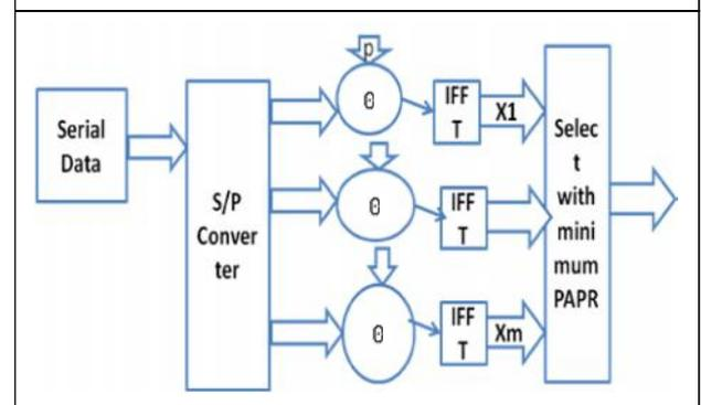
xd with the smallest PAPR is selected for final serial transmission.
