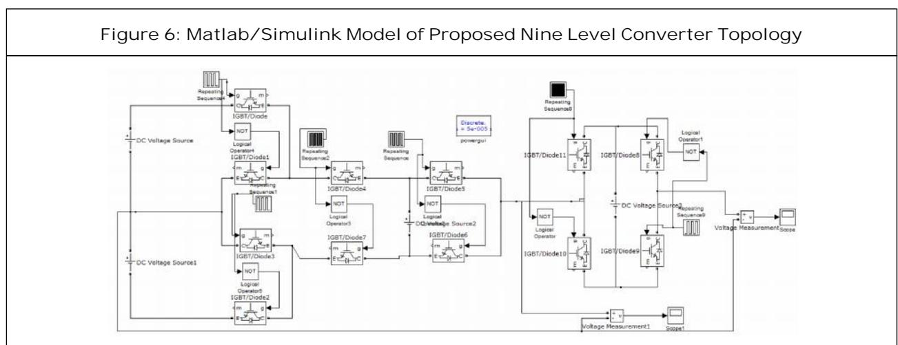
**Case 1: Proposed Nine Level Converter Topology for Grid Interconnection**
