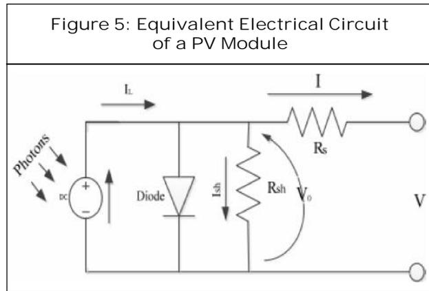
that equivalent circuit, a set of equations have been derived, based on standard theory, which allows the operation of a single solar cell to be simulated using data from manufacturers or field experiments.
