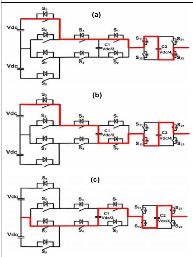
$$v_{out} = 0 + v_{c1} + v_{c2} = \frac{v_{dc}}{2} + \frac{v_{dc}}{4} = \frac{3v_{dc}}{4} \dots(8)$$
