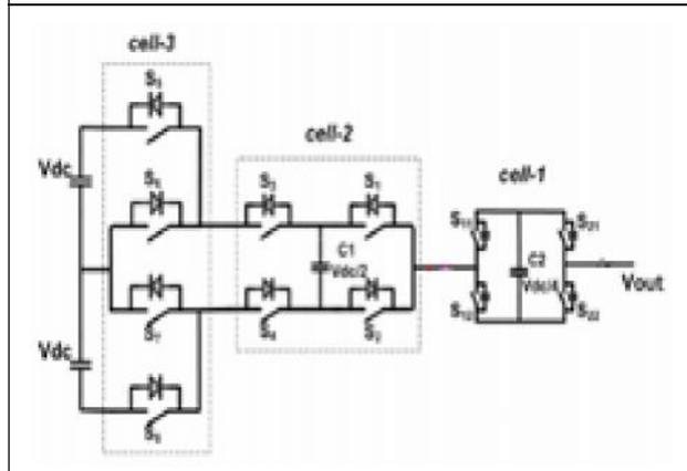
$V_{dc}/4$  for  $S_{11}$ - $S_{22}$ . Regarding the floating capacitors, their capacitance needs to limit the voltage ripple seen by the capacitors for a given switching frequency, which can be calculated by the following:
