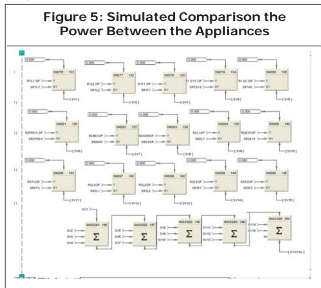
Under requirements of devices parameter are defined in the DCS as tag name which show in above simulation diagram.
