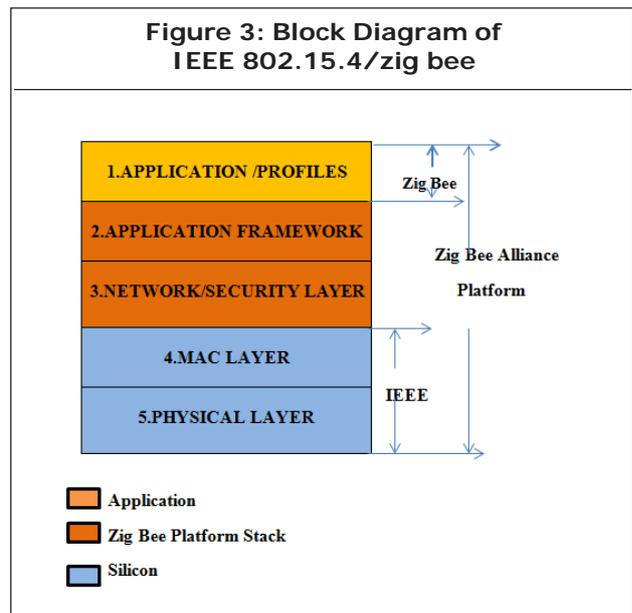
At the PHY layer, IEEE 802.15.4/Zig Bee uses Direct-Sequence Spread Spectrum (DSSS) with two different Phase-Shift Keying (PSK) modulations to minimize interference. At the MAC layer, Zig Bee adopts the CSMA/CA access to improve network throughput and minimize transmission delay.
