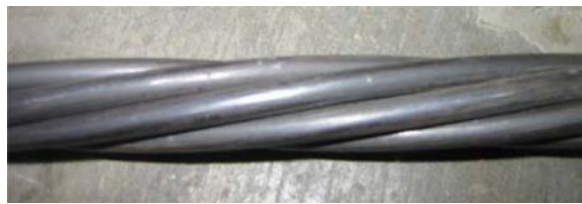
Figure 10: Strand After Exposure to 1000°F (538 °C)
