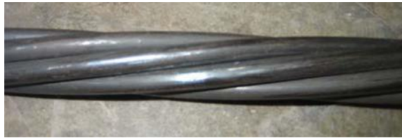
Figure 9: Strand After Exposure to 800°F (427 °C)
