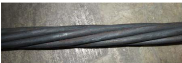
Figure 12: Strand after Exposure to 1300°F (704 °C)
