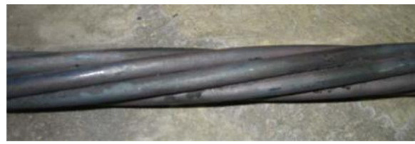
Figure 12: Strand after Exposure to 1300°F (704 °C)
