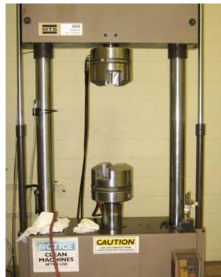
Figure 6: MTS880 Testing Machine Prior to Tension Tests
