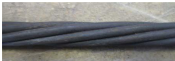
Figure 11: Strand After Exposure to 1200°F (649 °C)
