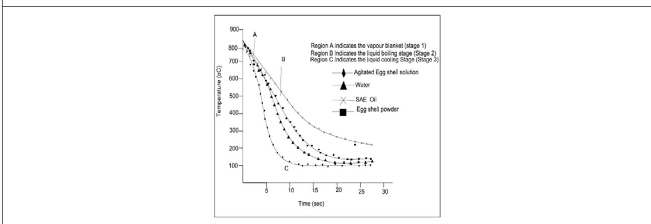
**Figure 5: Graph Showing the Cooling Rate of the Quenching Media**
