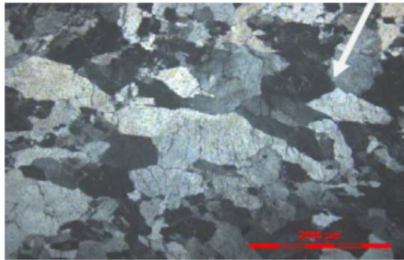
Figure 2: Alkali-silica gel extruded into cracks within the concrete
