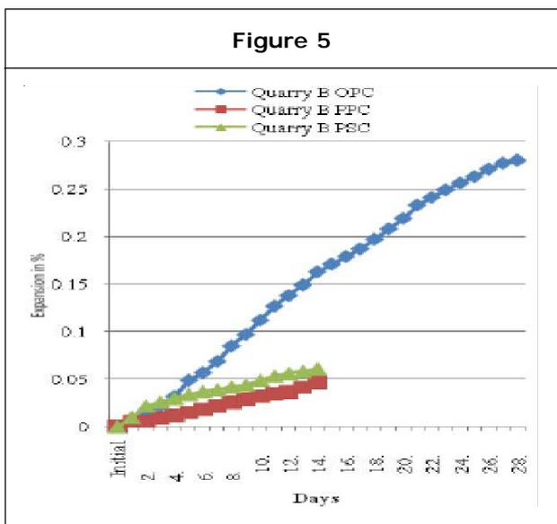
OPC while indicative of innocuous with both PPC and PSC. However use of PPC restricts the expansion due to ASR more than 14% in comparison to PSC at 14 days (Figure 5).
