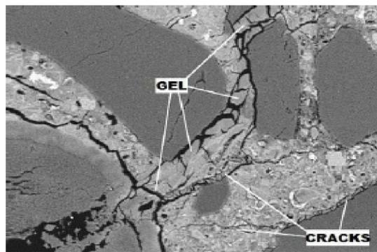
Figure 3: Aggregate particle with extending internal cracks due to ASR
