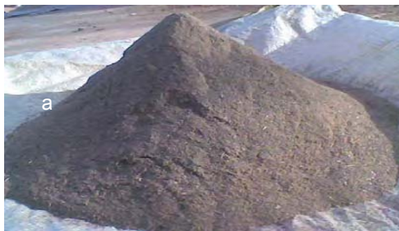
Figure 2: Photograph of (a) Coconut shell powder and (b) coconut shell ash
