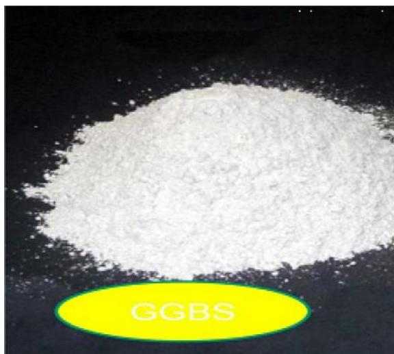
Ground granulated blast-furnace slag (GGBFS): Hydraulic cement formed when granulated blast-furnace slag is ground to a suitable fineness commonly referred to as slag cement, or GGBFS. In India, annual productions of pig iron is 70-80 million tons and corresponding blast furnace slag are about 21-24 million tons. The blast furnace slag could be used for the cement raw material, the roadbed material, the mineral admixture for concrete and aggregate for concrete, etc.
