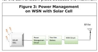
amount of energy needed for night time or dark shadow place and it's fully based on weather condition.
