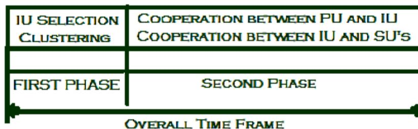
selected IU and cooperation is between the cluster head and other SUs in the cluster. The partner IU selection scheme is first performed, and then the cluster head IU cooperates with the PU in a TDMA manner that the PU transmits its package to the cooperating IU and the IU relays PU's last package to the BS simultaneously. After the cooperation between PU and IU, the IU finds the cooperative SUs who form a cluster from the surrounding starving SUs.
