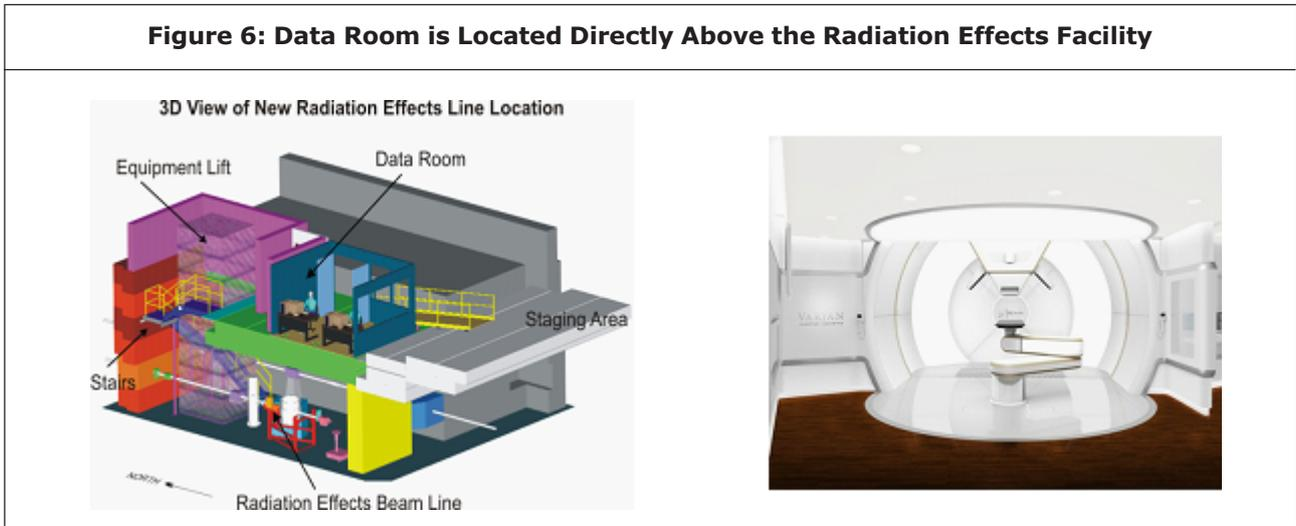
to provide the shortest distance possible between your equipment and your test board. From a table top in the data room to the top of the in-air station platter is approximately 15 feet.
