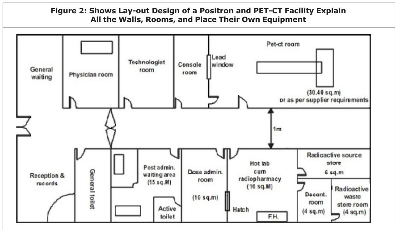
dimension of each of the rooms associated with the facility in the proposed layout plan of the NM department. When the user has to plan the laboratory, it is required that the arrangement of the various rooms associated with the facility has to follow the principle of low active area to high active area, that is, entrance of the facility should have reception/general waiting area, and at the end hot laboratory cum radiopharmacy/radioactive waste storage area is to be planned.
