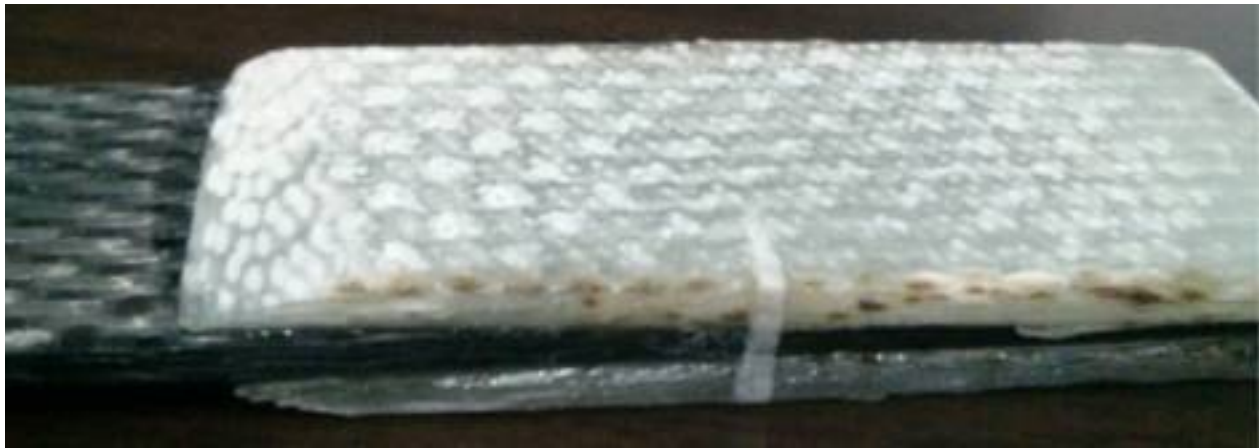
Figure 2: Glass Fiber Tabs Glued to the Specimen
