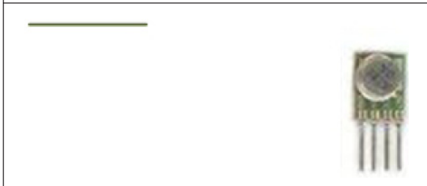
Figure 2: RF 434 Mhz Transmitter Modulation: ASK
