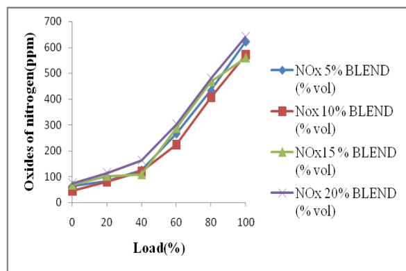
**Figure 13: Variation of Nitrogen Oxides Against Load at a Pressure of 2.9 Bar**
