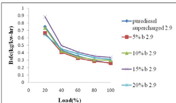
the load. The reason may be the extended ignition delay and the leaner combustion of biodiesel, resulting in a larger amount of fuel burned in the premixed mode of the ethanol blends.
