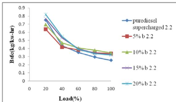
**Figure 9: Variation of Brake Specific Fuel Consumption Against Load at a Pressure of 2.9 Bar**
