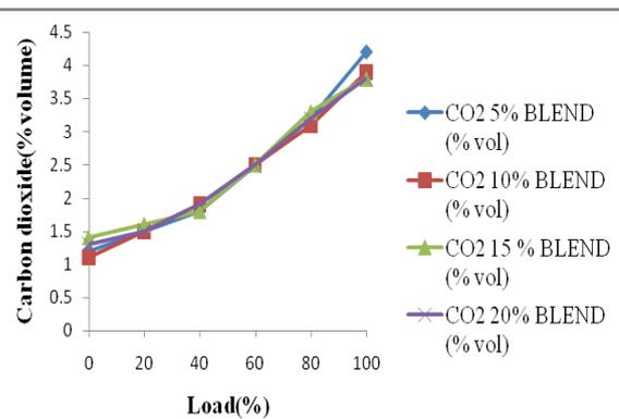
**Figure 15: Variation of Carbondioxide Against Load at a Pressure of 2.9 Bar**
