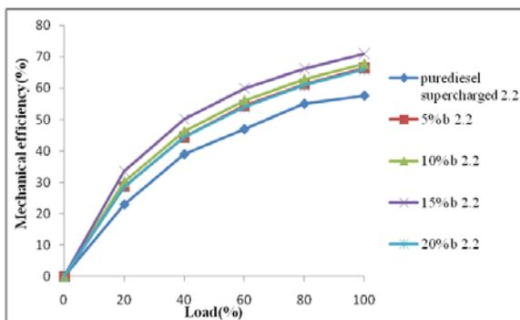
**Figure 5: Variation of Mechanical Efficiency Against Load at a Pressure of 2.9 Bar**
