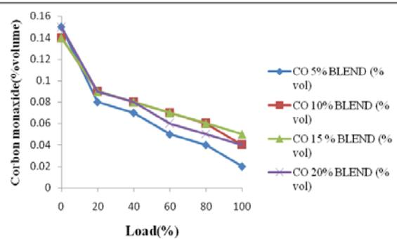
increase of percentage. The rice bran oil in the diesel at all loading conditions of the engine. It is due to the lower heating values of biodiesel compared with diesel fuel.
