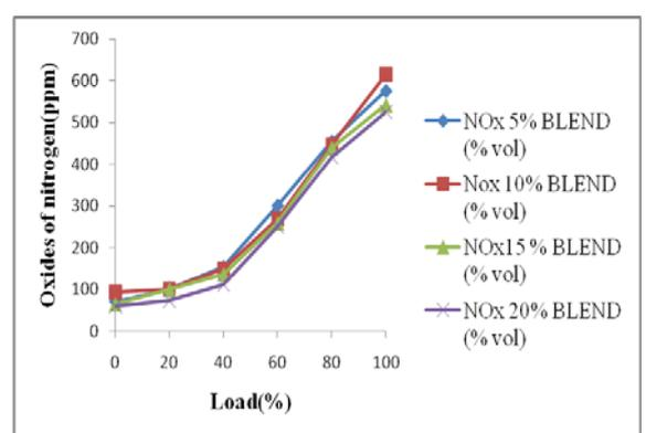
The variation of Oxides of Nitrogen (NOx) with load for biodiesel blends is shown in the Figures 12 and 13.
