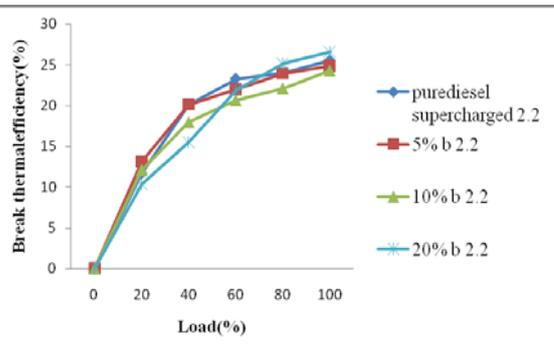
**Figure 7: Variation of Brake Thermal Efficiency Against Load at a Pressure of 2.9 Bar**
