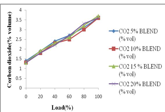
The CO<sub>2</sub> emissions increased with load for all the fuel modes. The CO<sub>2</sub> emissions of B5 at 2.2 abs, B15 at 2.2 abs, were slightly higher than the other blend. B10 at 2.9 abs and B15 at 2.9 abs were slightly higher than the other blends.
