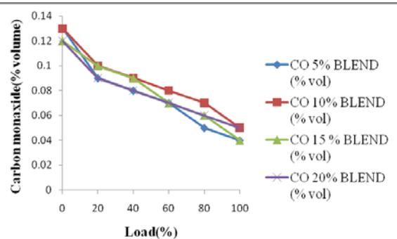
**Figure 11: Variation of Brake Carbon Monoxide Against Load at a Pressure of 2.9 Bar**
