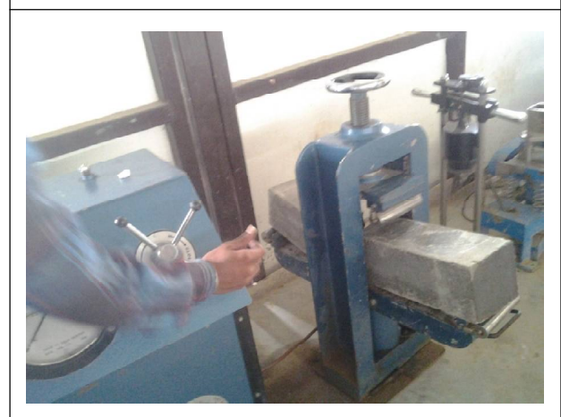
Figure 3: Photographic View of Flexural Strength Test
