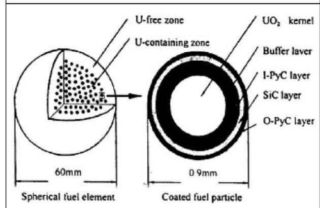
particles. Each fuel particle consists of a UO<sub>2</sub> kernel, which is coated with four layers. These are; low-density pyrolytical carbon, inner high-density pyrolytical carbon, silicon carbide and outer high-density pyrolytical carbon layer. The uranium content per fuel element will be 5 gm with U-235 enrichment of 17% (Sen *et al.*, 2001; IAEA TECDOC 1382, 2003; Hu *et al.*, 2004; and Tiawo *et al.*, 2005).
