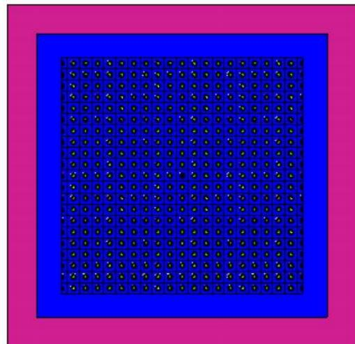
TRISO particle is composed of 5 layers. The sphere in the heterogeneous model is converted into a rectangular form with volume and mass conservation for all materials. Model B is shown in Figure 3.
