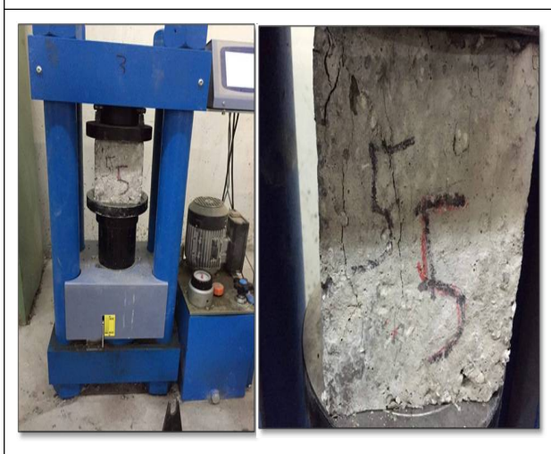
Figure 4: Compressive Strength Test
