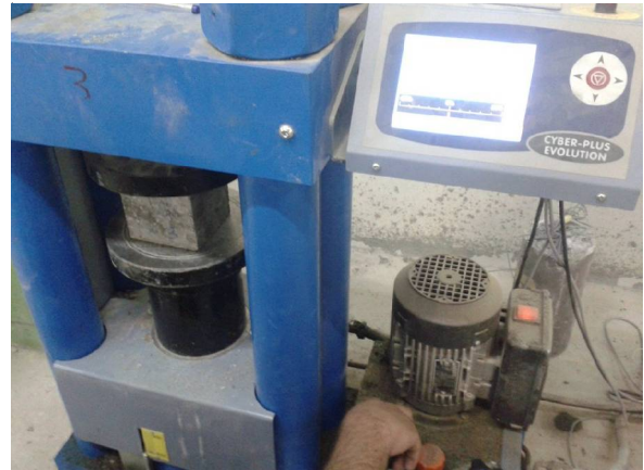
Figure 3: Compressive Strength Test
