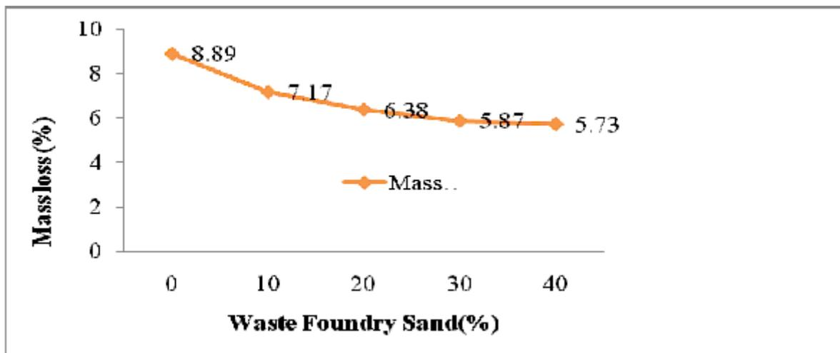
Figure 13: Mass loss (56days) of Concrete Specimen Due to Immersion in 5% H<sub>2</sub>SO<sub>4</sub> Solution
