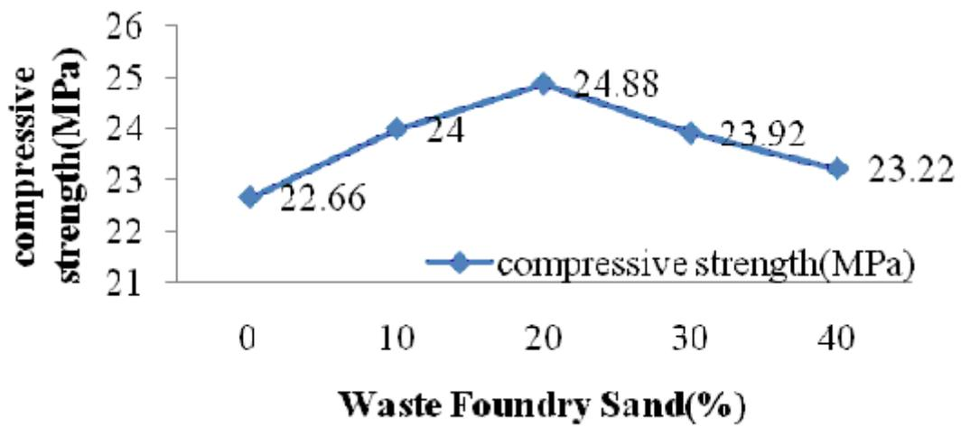
Figure 3: Compressive Strength vs. Replacement of Waste Foundry Sand at 28-days
