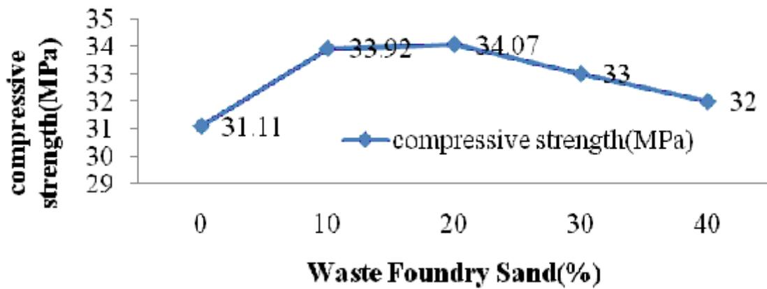
Figure 4: Compressive Strength vs. Various Replacement Levels of Waste Foundry Sand Split Tensile Strength
