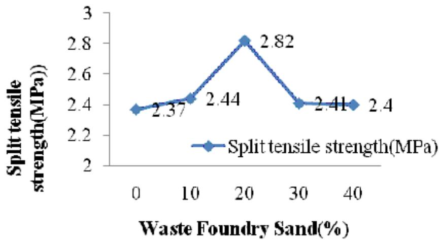
Figure 6: Split Tensile Strength vs. Replacement of Foundry Sand at 28-days
