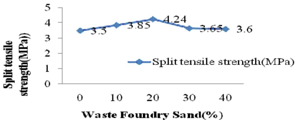
Figure 7: Split Tensile Strength vs. Various Replacement Levels of Foundry Sand
