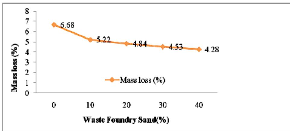
Figure 12: Mass loss (28days) of Concrete Specimen Due to Immersion in 5% H<sub>2</sub>SO<sub>4</sub> Solution
