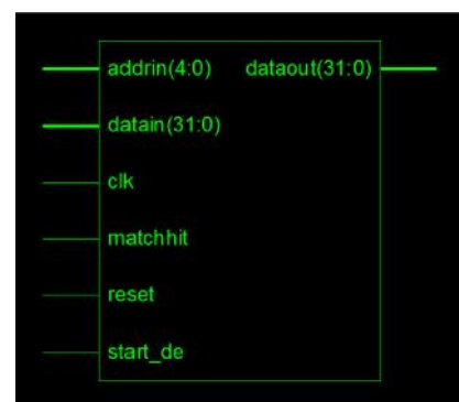
Figure 9: The RTL Schematic for De-compression Using Xilinx
