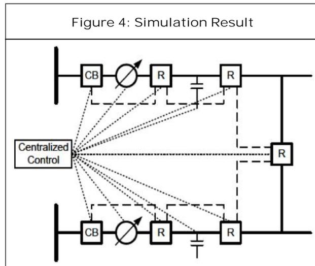
useful when coordinating a large or very diverse distribution system. Peer-to-peer systems become more complex as more interconnections or multiple sources are added to the system. Figure shows a centralized control system used for automation. Protection functions should still be addressed locally in each device or using high-speed peer-to-peer communications.
