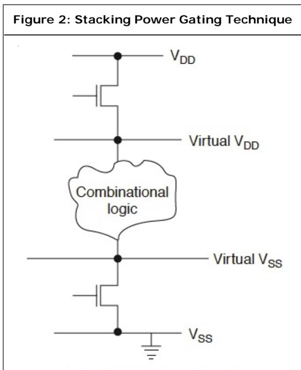
header switches to shut off power supplies, the stacking Power Gating parts of a design in the mode of sleep or standby. NMOS footer switches can also be used as sleep transistors in the design of stacking power gating technique. The
