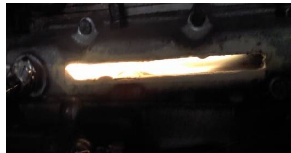
Figure 7: Propagation Flame Heaters in the Intake Pipes of Diesel Engines DM34 with Euro Diesel
