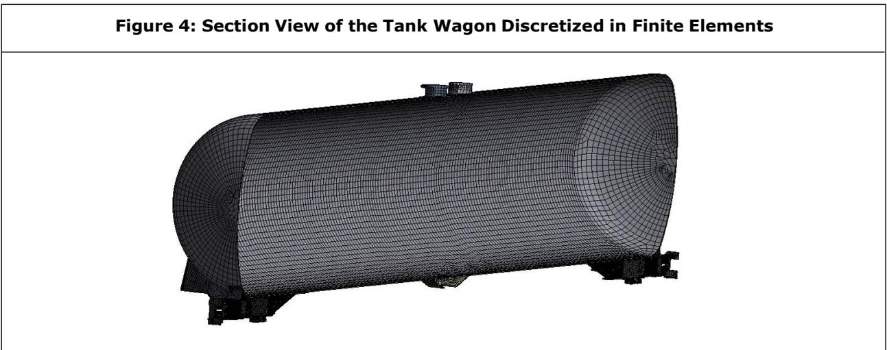
presence of the fluid, the pressure was directly applied to the inner walls of the shell with a fluid density of 1000 kg/m<sup>3</sup>, which is slightly larger than of the tank cars intended for the transportation of hydrocarbons. The boundary conditions provided by the trucks were simulated by using simple supports at each end. This configuration can be seen in the diagram of Figure 5.
