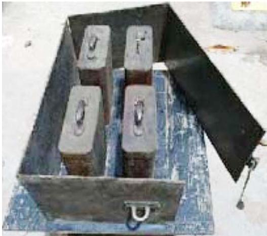
rectangular steel mould and inserts onto the wooden plank. Two patterns of hollowness were introduced one with two rectangular holes and another pattern with four holes as shown in Figure 6 and 7. The size of inserts for a 2 holed block were 100 mm x 125 mm x 200 mm and that of 4 holed were 145 mm x 45 mm x 200 mm with both inserts uniformly tapering at the bottom by 1 cm.
