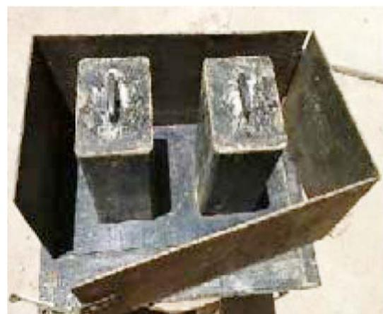
**Figure 7: 4 Hole Hollow Block Fabricated Mould**
