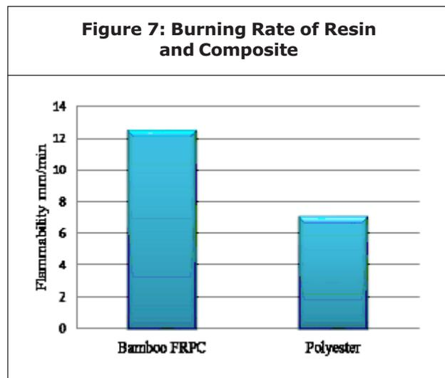
The burning rate of bamboo/polyester and sisal/pp composites is almost doubled while LDPE/AB wood composite is lowered to half (Table 3).
