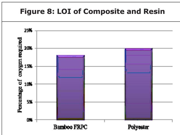
The limiting oxygen index bamboo/polyester composite is compared with coconut/PLA and wood/PP and noticed that bamboo/polyester composite burns easy comparatively (Table 4).
