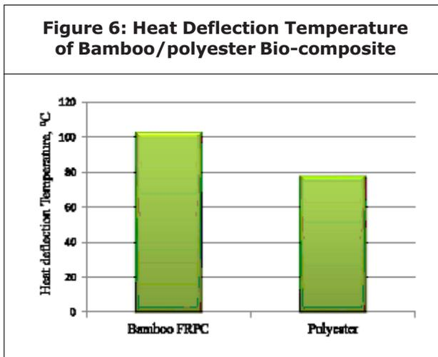
The HDT of Bamboo FRPC is compared with the Kenaf/PLA composite and Banana/PLA composite in the Table 2. Kenaf/PLA composite showed a drastic increase in HDT value only with fiber volume fraction of 0.1 while the composites HDT values are not so remarkable.
