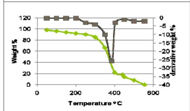
**Figure 5: DGA Curve for Polyester Resin**
