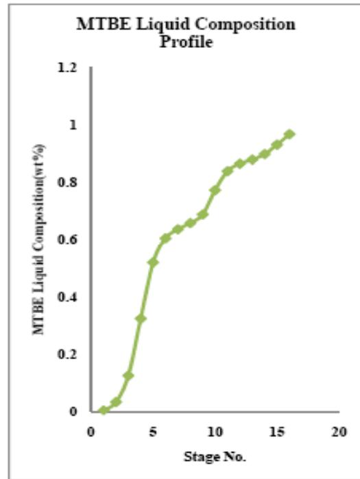
50% vaporized feed is fed to the column. It can be observed from this graph that the MTBE composition increases from the top to the bottom of the column. It is almost in negligible amount in the top and maximum amount of it is present in the bottoms, almost 97%, which can be attributed to its higher boiling point. It is desirable also to get maximum amount of MTBE in the bottom of the column in as much as pure form.
