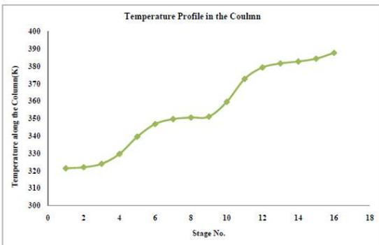
Figure 9 shows the temperature variation along the column, when a 50% vaporized feed is fed to the column. It can be observed from this figure that temperature increases from top to the bottom of the column. It shows the same pattern as for the saturated liquid feed, however, the variation of the temperature near the feed stage is found
