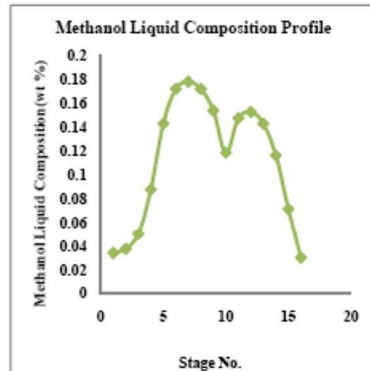
Figure 2 shows the variation of methanol composition inside the column. As can be seen from this graph, two methanol concentration peaks occur inside the column in the liquid phase, one above the feed tray and one below the feed tray. Figure 3 shows the variation of MTBE (Methyl
