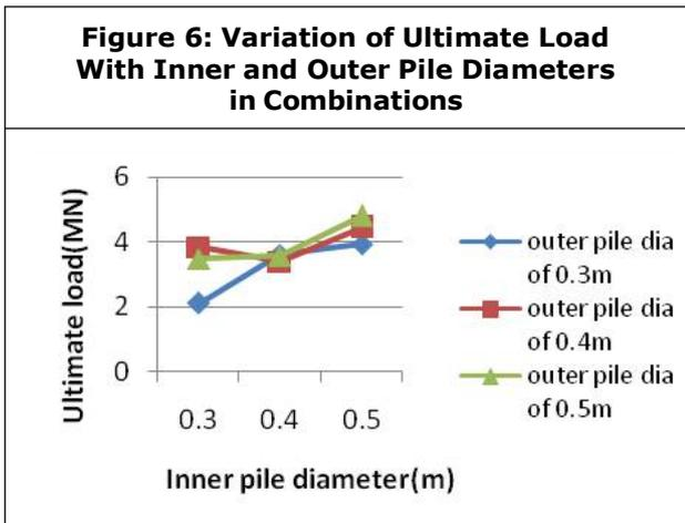
From the above results, a pile diameter combination of 0.5 m at the centre of the raft with 0.4 m at the edge of the raft is showing credible results.
