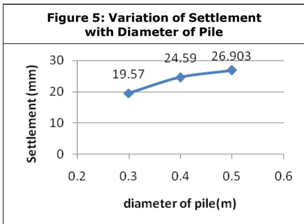
The ultimate load carrying capacity and corresponding settlement is obtained for piles of different diameters in different combinations are discussed in the following (Table 3).
