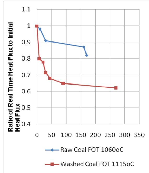
**Figure 6(c), 6(d): Comparison of Heat Flux Reduction for Raw and Washed Coals at Around 850°C for Burner Zone and Furnace Exit Panels**
