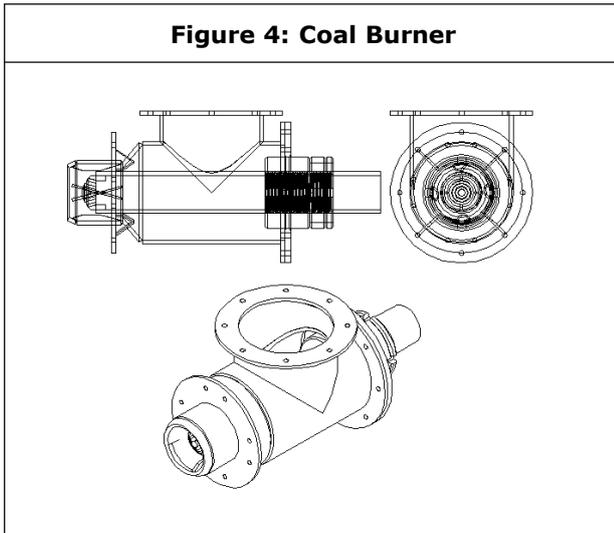
fire air. The burner nozzle is designed in such a way that the fuel-air mixture can flow at any pre-determined velocities representing low, medium and high velocity ranges depending upon the volatile content of coal.
