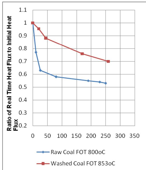
However, since the absolute values of heat fluxes are higher in the burner zone and on washing the heat absorption is improving in that zone the net effect on the furnace is likely to be better on use of washed coal.
