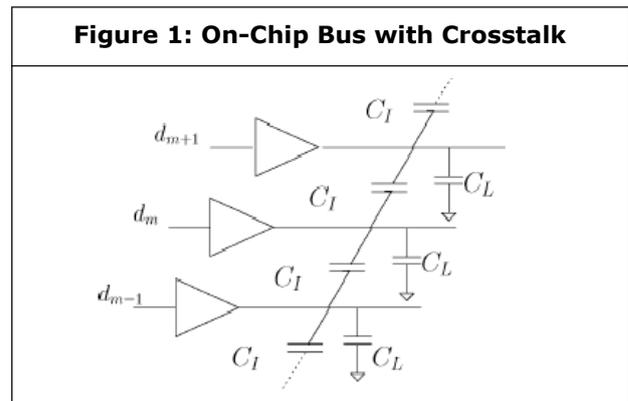
**Figure 1: On-Chip Bus with Crosstalk**
