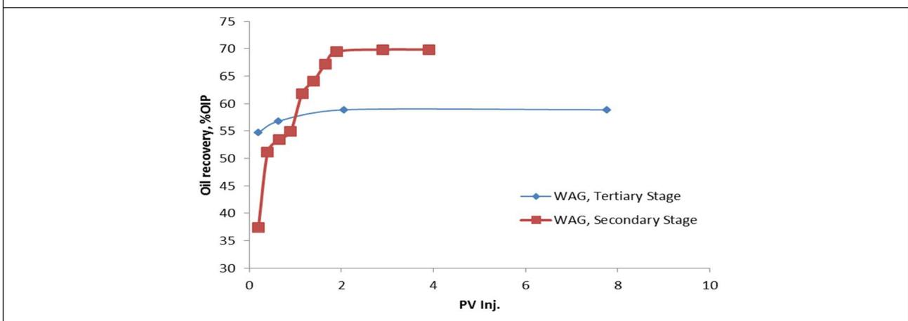
**Figure 15: Displacement Efficiencies of Secondary and Tertiary Schemes**
