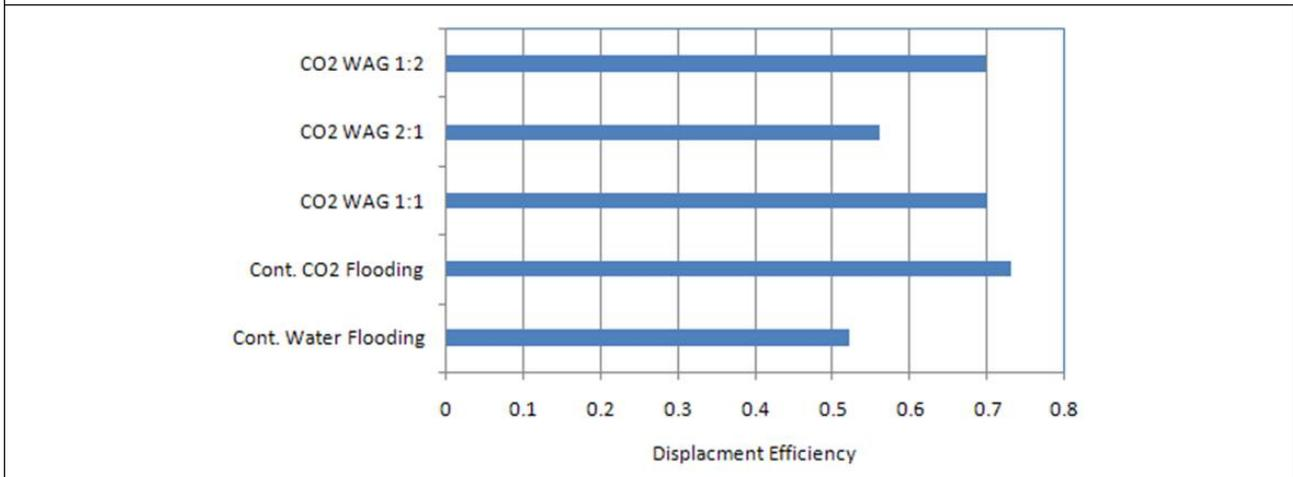
an acceptable alternative for CCGI and the optimum CO<sub>2</sub> flooding system for the selected field. On the other hand, WAG 2:1 and Continuous brine injection came in last in this comparison.
