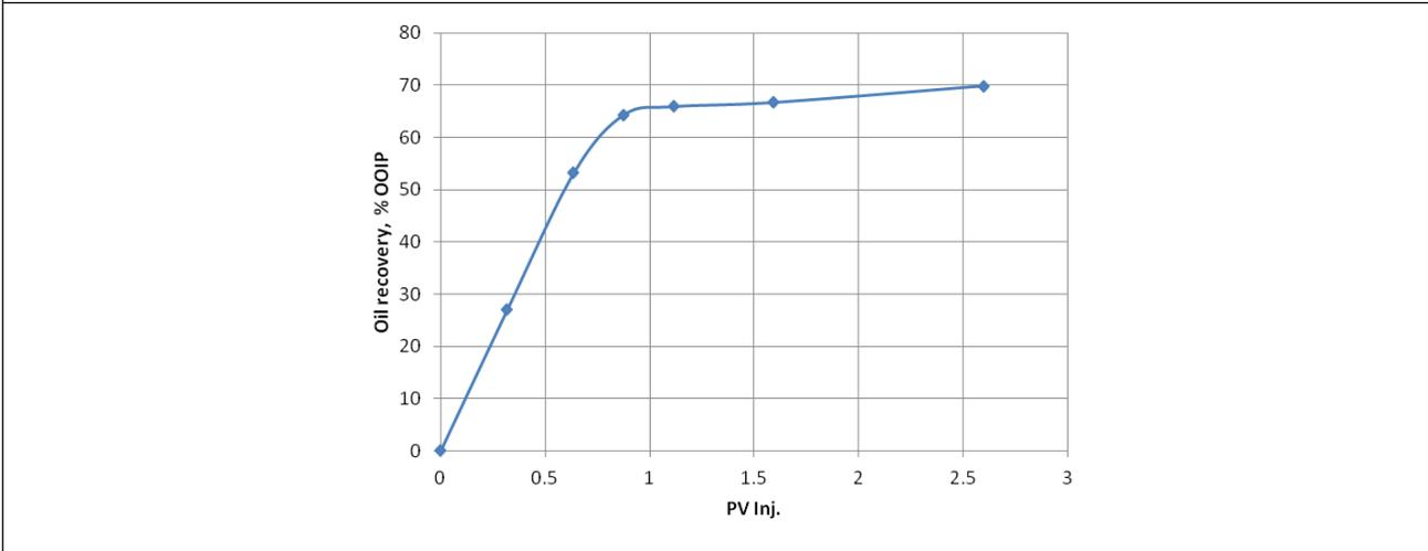
**Figure 7: Experimental Results of WAG Ratio 2:1 in Secondary Recovery Scheme**
