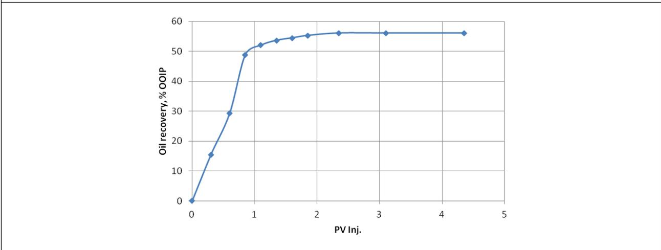
**Figure 8: Experimental Results of WAG Ratio 1:1 in Tertiary Recovery Scheme**
