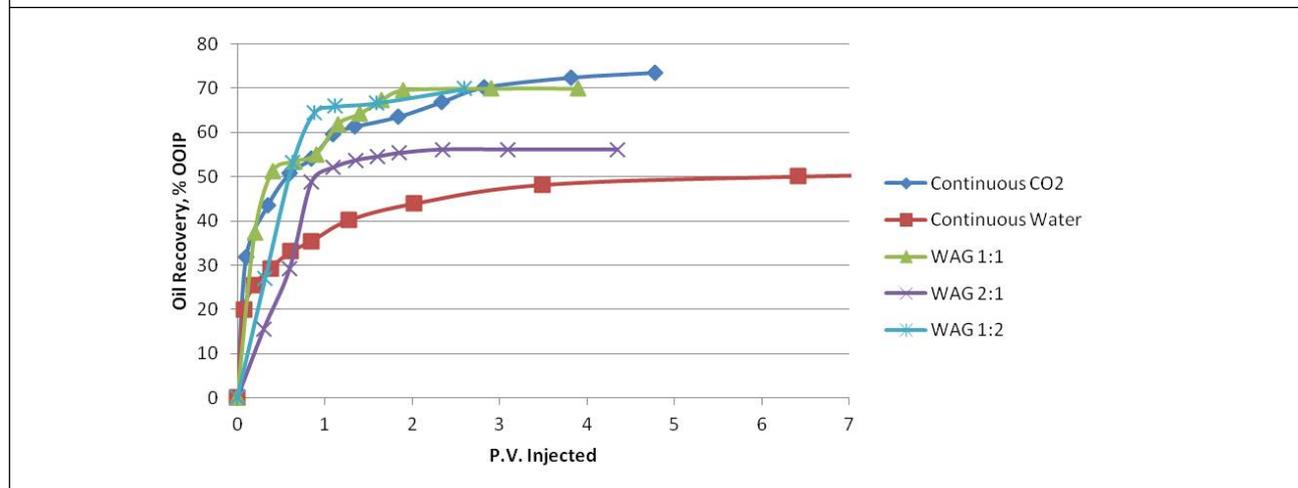
**Figure 13: Displacement Efficiencies by Various Flooding Methods**
