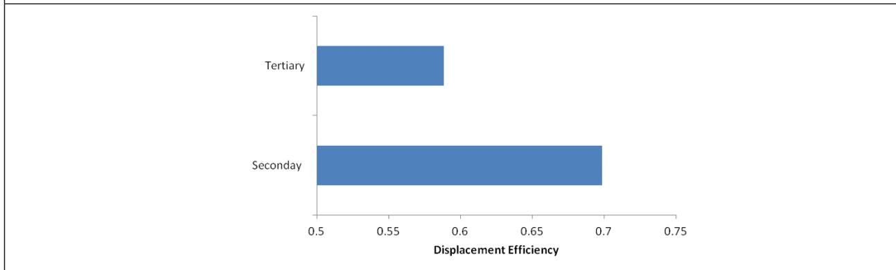
which shows that secondary mode has a value of 0.7 with only 0.59 in the case of tertiary stage of production.
