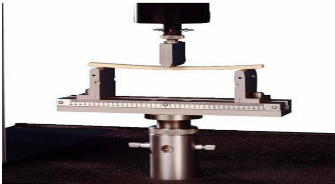
Figure 1: Three Point Bending Fixture
