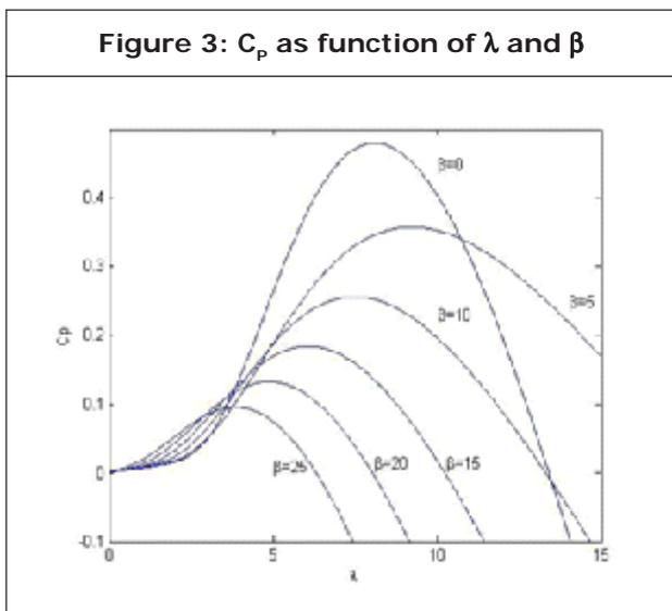
$$C_p(\lambda, \beta) = C_1(C_2 / \lambda_i - C_3\beta - C_4)e^{-C_5/\lambda_i} + C_6\lambda_i \quad (3)$$
