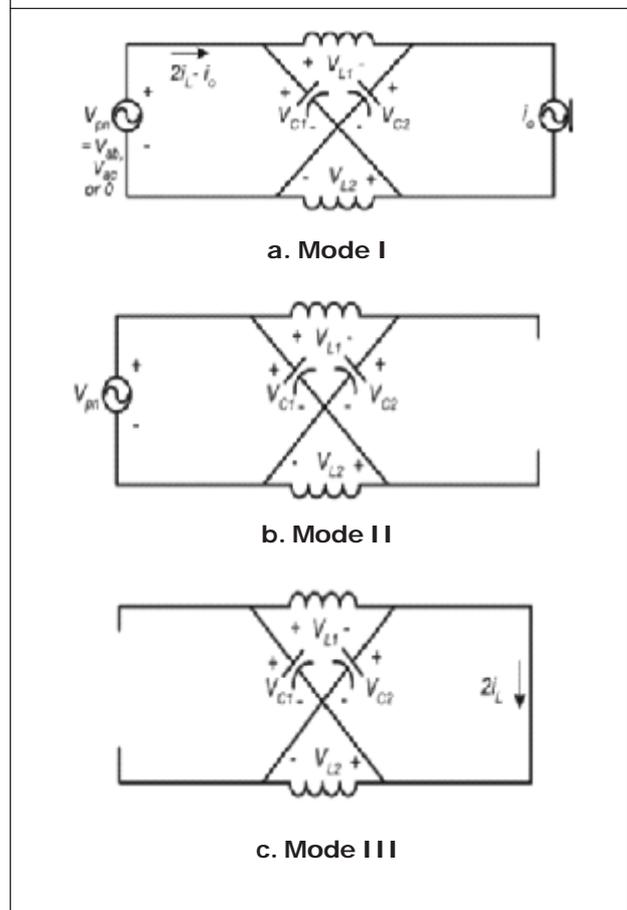
Mode I: Operates in one of the six non-zero vectors, thus acting as a current source when viewed from Z-source network. Therefore the current in the inductor is symmetric.
