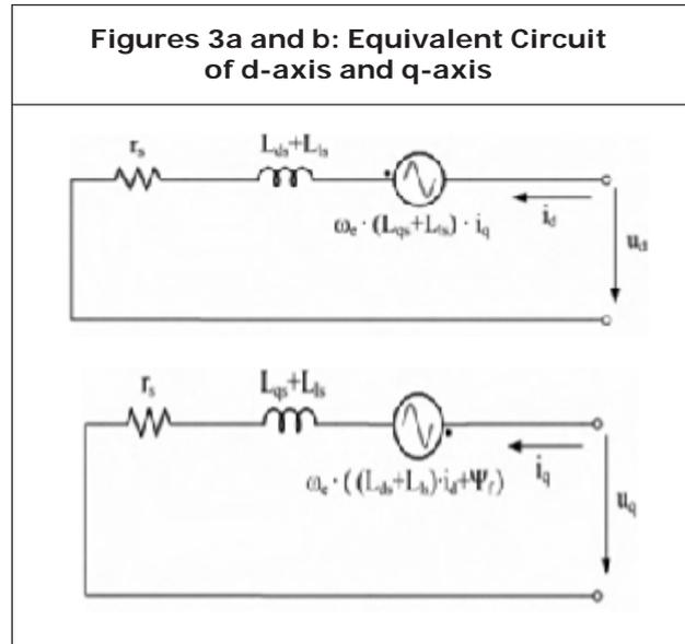
The model of the PMSG is obtained from the two pole synchronous reference frame, which the 0.q-axis is 90° ahead of the d-axis with respect to the direction of rotation. It is illustrated by the following equations;
