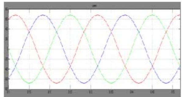
**Figure 10: NPC inverter output voltage**
