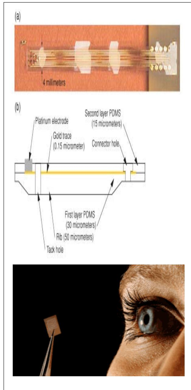
between two layers of PDMS. Reinforcement ribs facilitate handling of the thin PDMS device. A tack hole is used to pin the device to the retina.
