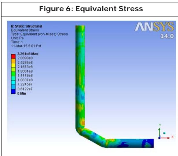
Figures 4,5,6,7 shows the total deformation, directional deformation, equivalent elastic strain equivalent stress at  $\phi_1 = 120^\circ$  and  $\phi_2 = 150^\circ$ ,  $\psi_1 = 60^\circ$  and  $\psi_2 = 30^\circ$  angles in ECAP die.
