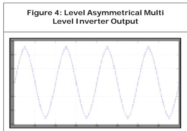
1 bridges and approximately 3% of the total power from Aux-2 bridges. All bridges have their input voltage source. They all are in the GP ratio 3. MOSFETs are used as switches. All the bridges are switching at different frequencies. The MAIN Bridge operates at fundamental frequency while the other two AUXILLARY bridges are operated at higher than fundamental frequencies.
