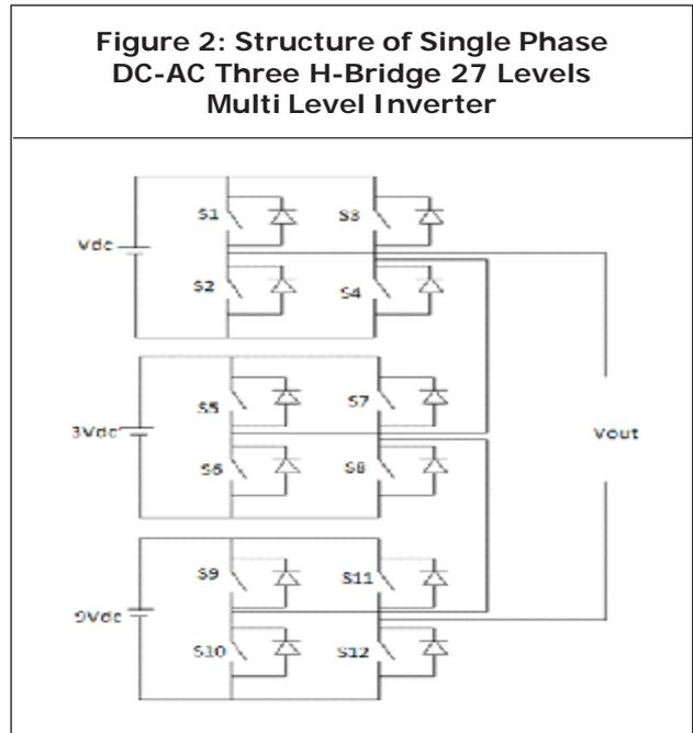
sources inverter, each bridge having separate dc sources and different amplitude of voltage. These supplies are fed to different combinations of switches. The output of each bridge is fed series with each other. In 3 H-bridges MLI, the final output can be obtained from 1<sup>st</sup> and 3<sup>rd</sup> bridges as shown in figure 2.
