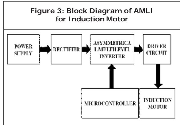
DC. The DC power is fed to asymmetric MLI (AMLI). The AMLI is converts the DC power into controlled AC power. The microcontroller is used to generate the gate pulse. These gate pulses of Microcontroller is fed to the switches of AMLI through the driver circuit to drive the induction motor.
