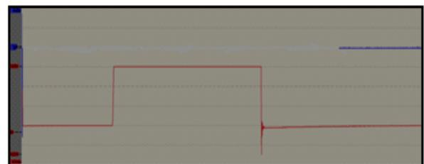
From the phase comparator simulation output, the voltage is high if the per phase of inverter is same with per phase of line grid. After the delay of 40 millisecond of output inverter, the result of
