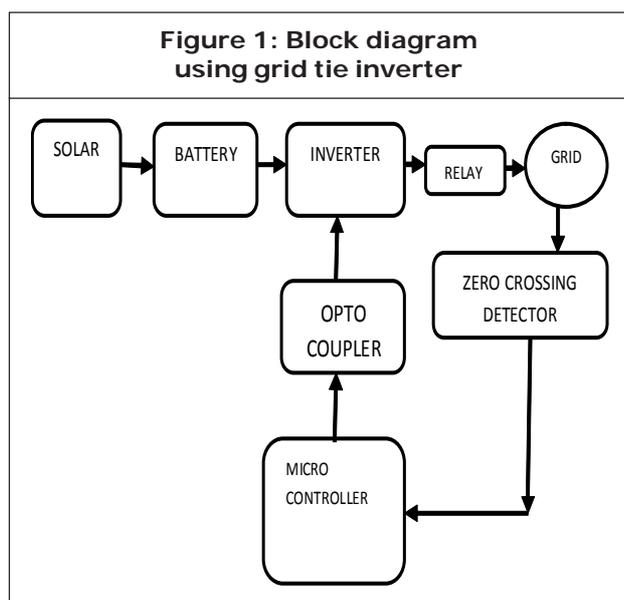
models of a grid-connected PV system. PV array is connected to the utility grid by DC/AC inverter. zero crossing detector is used to avoid deviation between inverter and grid and synchronization is carried out.
