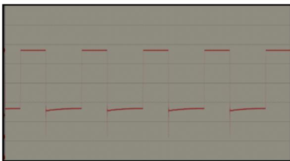
For the voltage comparator circuit, the simulation shows that the comparator take about 76 millisecond to becomes high(5 volt) after being feed with 40 millisecond delay of PWM inverter output.
