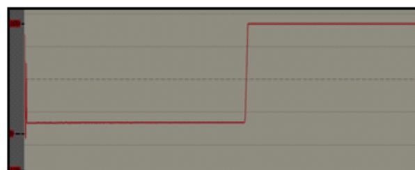
phase comparator shows that the output voltage become high(5 volt) after 42 millisecond. It means that the comparator its self only take 2 milliseconds delay to operate
