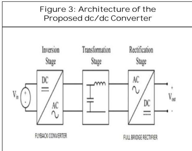
The inversion stage is designed using a fly back converter. Proposed converter design is shown in Figure 4. It consists of a dc supply from a battery source. It is given to a flyback converter
