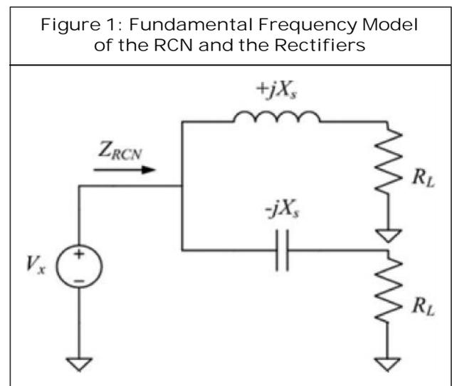
Although the structure (called resistance compression network) is simple and significant suppression of the load variations is possible, the structure is only applicable to DC-DC conversion systems, where the same effect could be achieved if the active solution had been pursued instead. Compression networks ideally act without loss, such that all energy provided at the input port is transformed and transferred to the resistive load. In effect, the load resistance range
