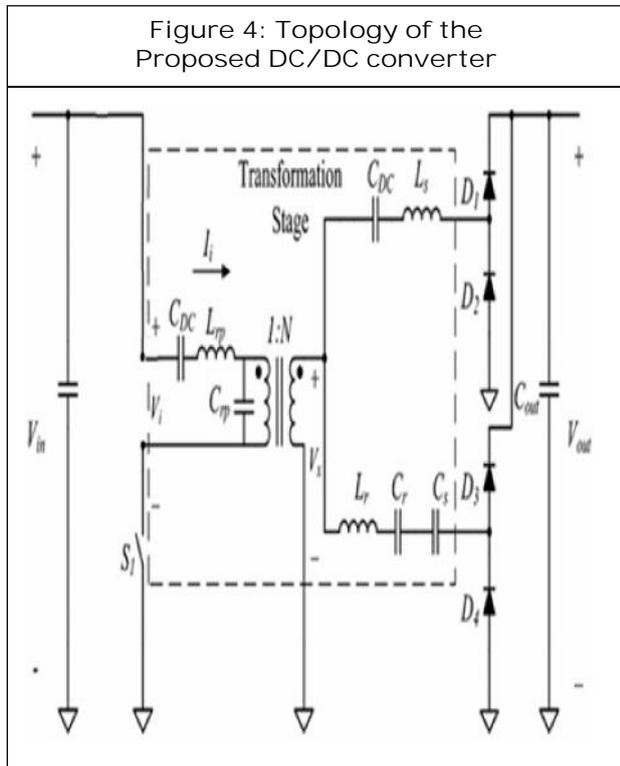
which consists of a MOSFET switch and a flyback transformer. The transformation stage includes a resistance compression network (RCN) and filters. Then followed by a two half bridge diode rectifier. This rectifier supplies the load. The operation explains the working design of the converter.
