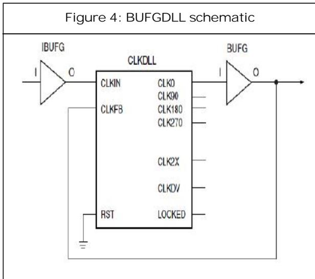
This symbol does not provide access to the advanced clock domain controls or to the clock multiplication or clock division features of the DLL. This symbol also does not provide access to the RST, or LOCKED pins of the DLL. For access to these features, a designer must use the library DLL primitives described in the following sections.
