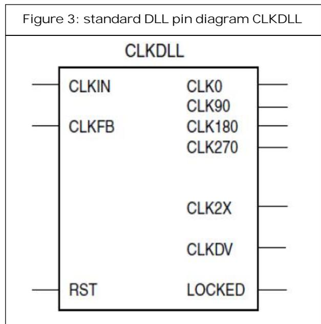
Figure 3: standard DLL pin diagram CLKDLL
